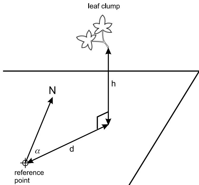
FIG. 4.1 – Method to measure the location of leaf clumps. Leaf clump base is characterized by its height  $h$ , distance  $d$  from a reference point, and angle  $\alpha$  from a reference direction (e.g. North).
