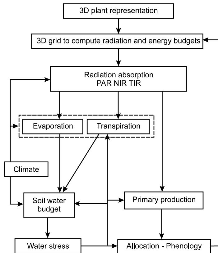
FIG. 6.1 – Processes computed in the TREEGRASS model
