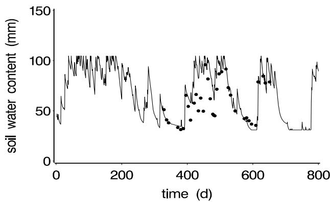
FIG. 6.6 – Measured (●) (Le Roux 1995) and simulated (lines) seasonal courses of soil water content in the upper layer (0-60 cm) under a tree clump, during two annual vegetation cycles.
