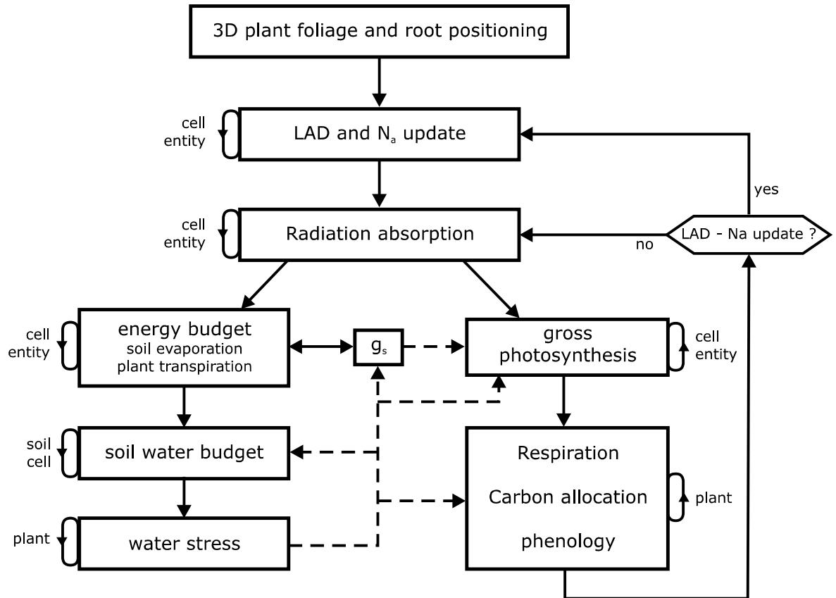
FIG. 7.1 – Main processes computed in TREEGRASS-2. Plain lines correspond to the flow chart. Dashed lines represent effect of water stress occurring the following time step. Loop level is indicated (plant, soil cell, or entity in each 3D grid cell, i.e. leaf type or soil surface). Leaf area density (LAD) and leaf nitrogen per unit leaf area ( $N_a$ ) are updated in the 3D cell grid when a threshold variation has occurred.
